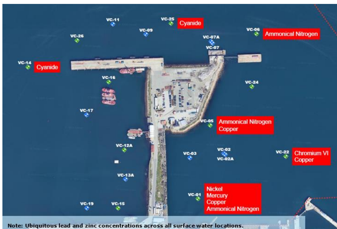
Figure 8: March 2024 Ground Investigation Summary of Surface Water Exceedances Across the Site
